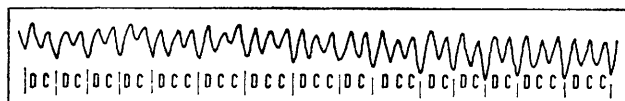
FIGURE 7 Microphotometer trace across A–A' showing lamella of D–C–C–D–C–C–D– stacking, corresponding to \text{Nb}_{39}\text{O}_{97}
